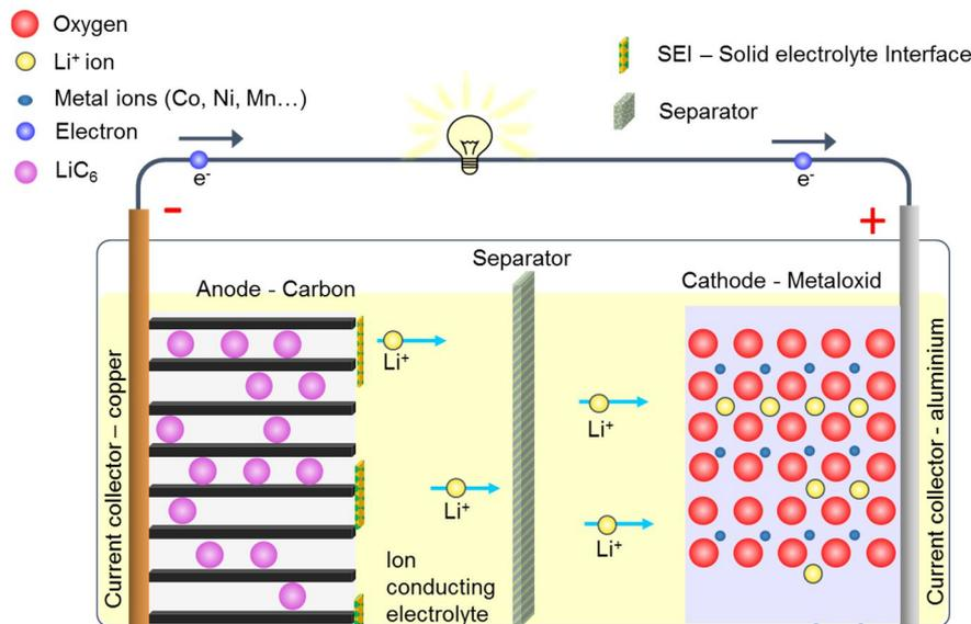
Figure 1: Lithium-ion battery cell during discharge
