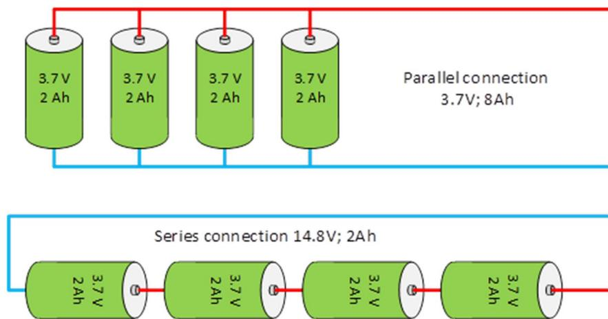
Figure 4: Series and parallel connections of cells.
