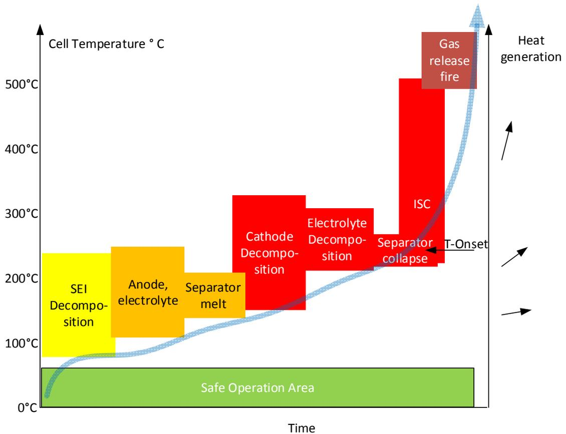
Figure 3: Thermal runaway events at different temperatures.
